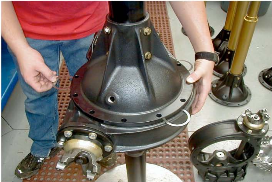
Spacer shims are placed between the center section and the right bell to adjust for crush clearance. This is a trial-and-error way to obtain the correct shim spacing behind the differential bearing to arrive at 0.010-inch crush when tightening the bell to the center section.
