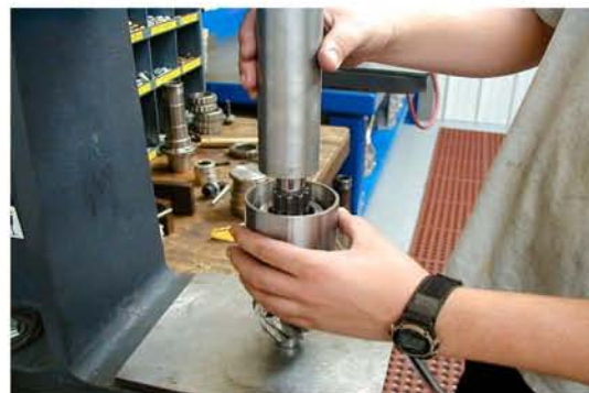
Special tools are used to press the bearings onto the pinion shaft. These ensure that the bearing goes on straight and is properly seated.
